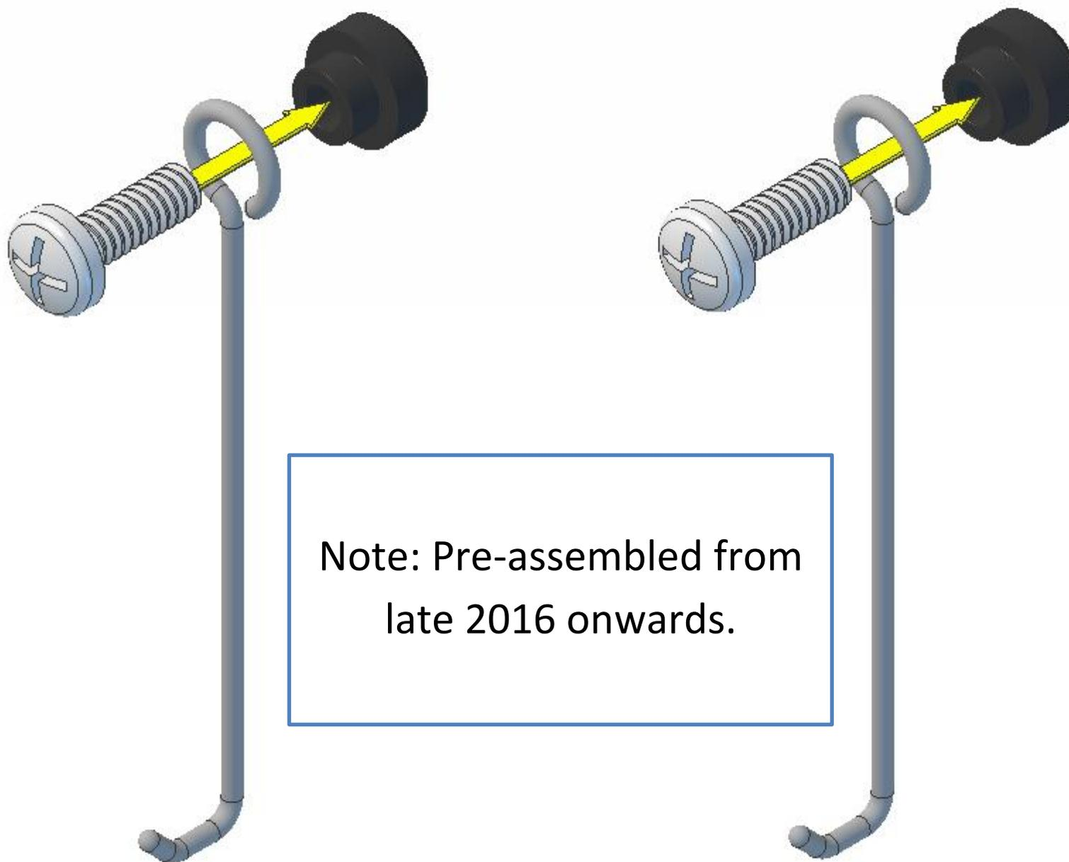
Screw the screws in until they *just* touch the bushes. Do not over-tighten or you could cause the bushes to expand and pinch the conrod eyes, which could prevent your engine from running.
