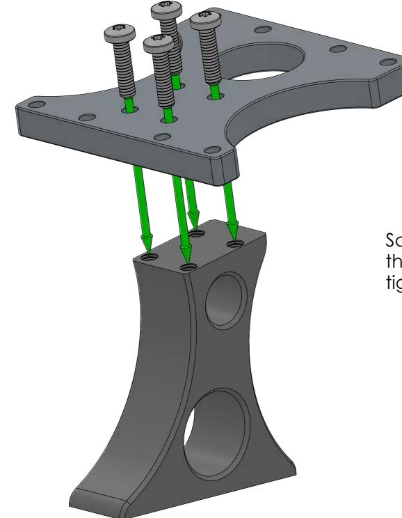
Screw four M2x8 screws through the foot bracket into the foot and tighten.
