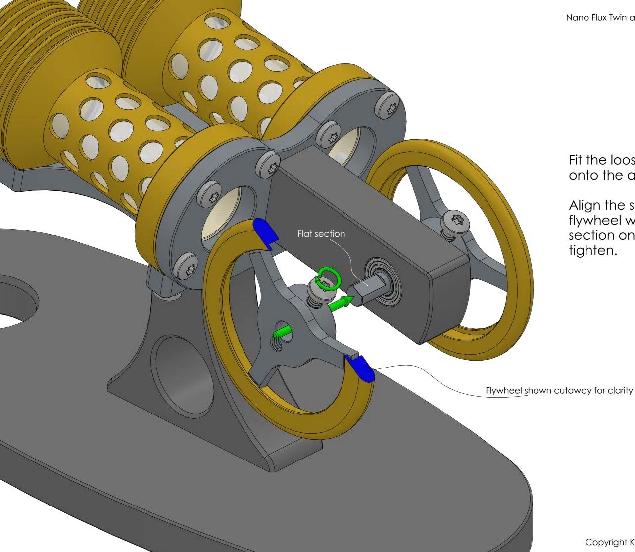
Fit the loose flywheel onto the axle.
