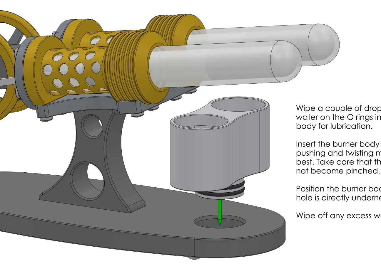
Wipe a couple of drops of soapy water on the O rings in the burner
