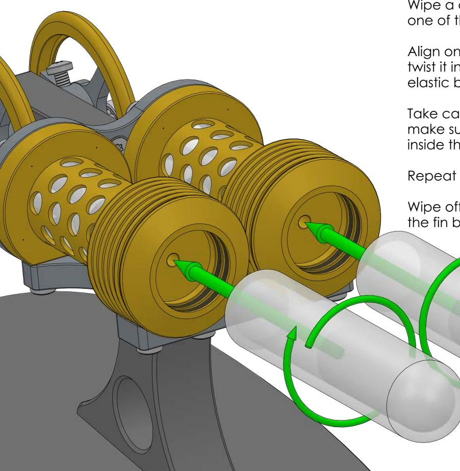
Wipe a couple of drops of soapy water on the O rings in one of the fin blocks for lubrication.
