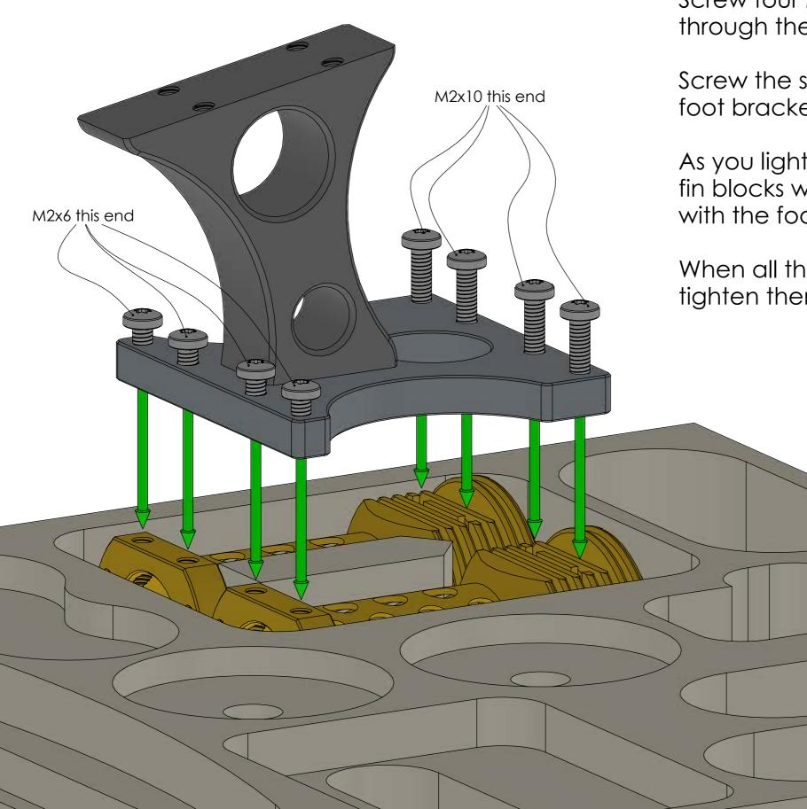
Screw four M2x10 screws and four M2x6 screws through the foot bracket into the fin blocks.
