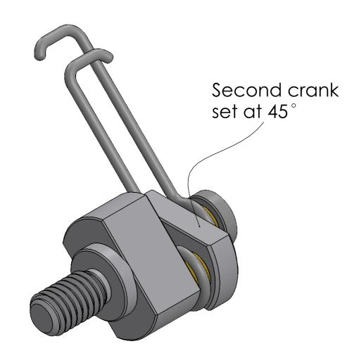
To reset the angle slacken the crank screw slightly (1) and fit the crankset into the crank angle tool as shown.
