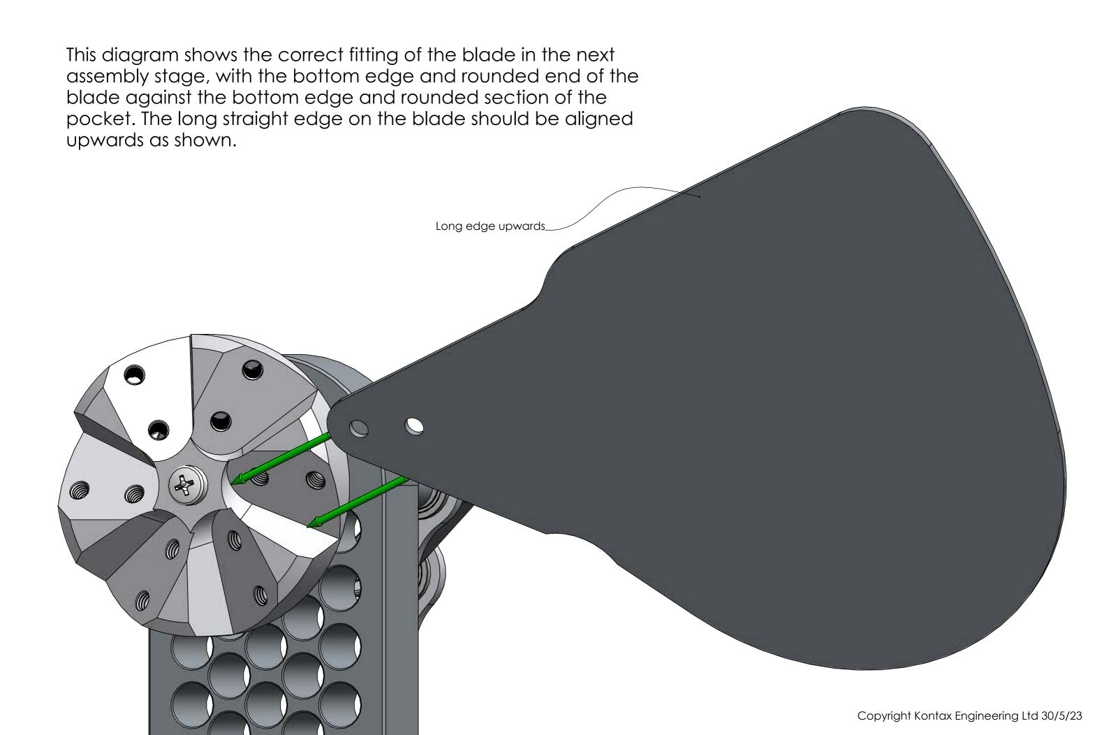
With the blade positioned as shown on the previous page screw the first short screw through the hole in the blade and into the hub so that it just holds the blade lightly, and then screw the second screw in the same.
