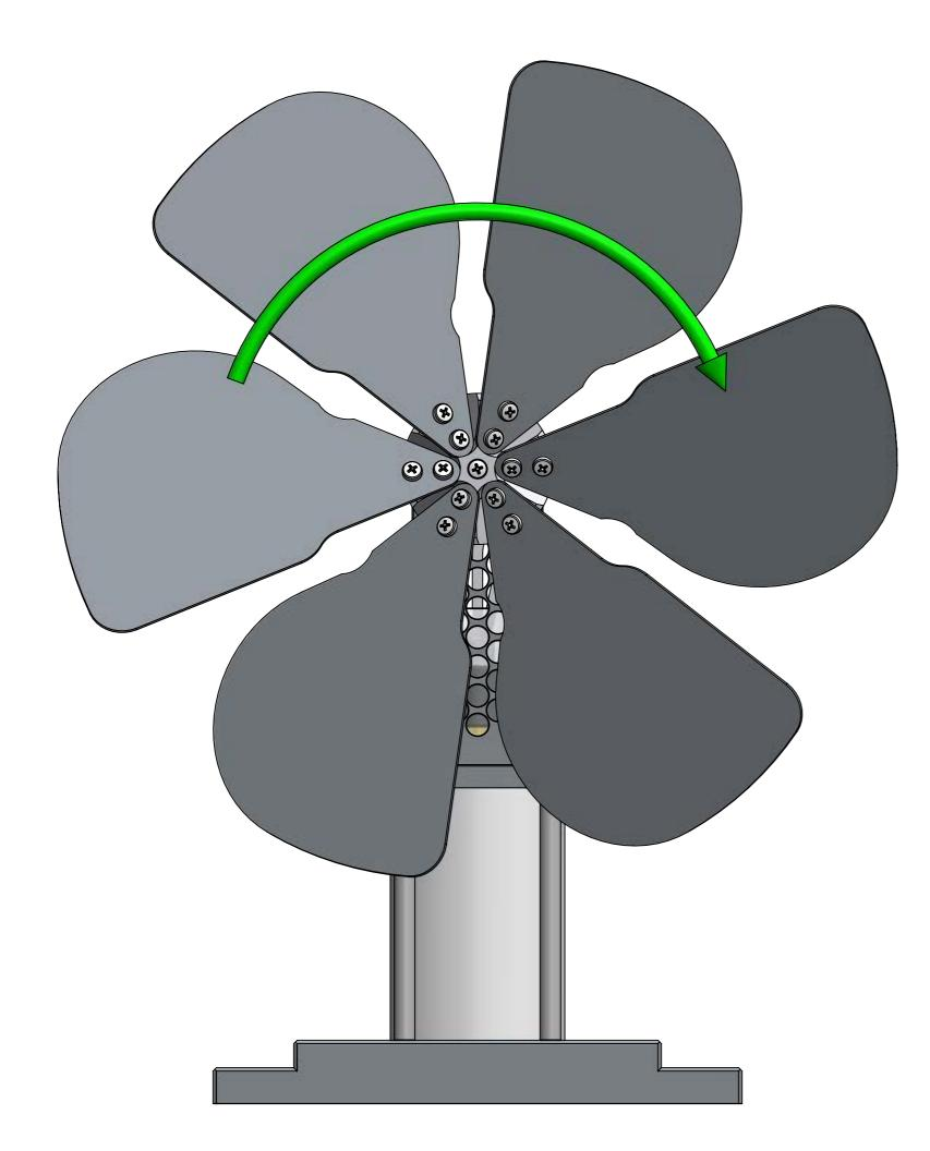
The fan has been factory-set and tested to run at over 400rpm at 350°C.
