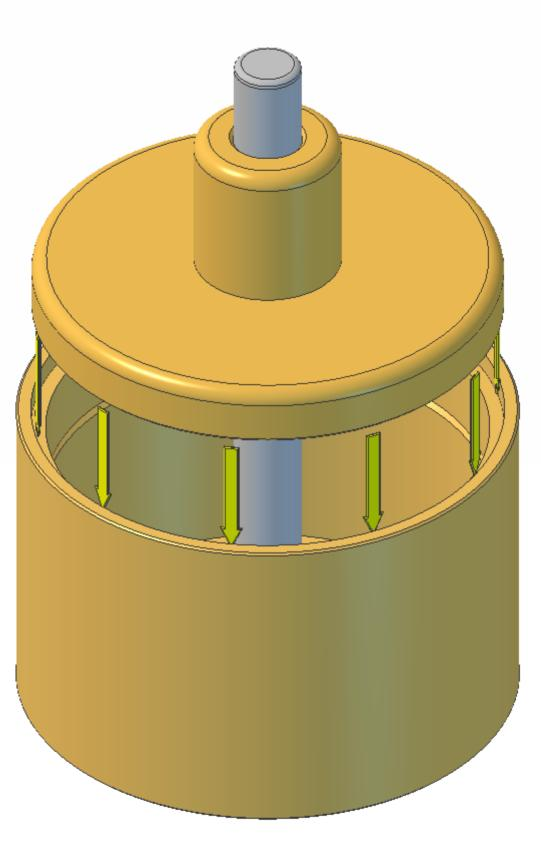
Fit the assembled burner into the hole in the plate.
