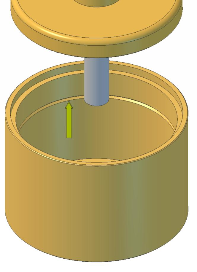
Fit the burner cap into the burner body.
