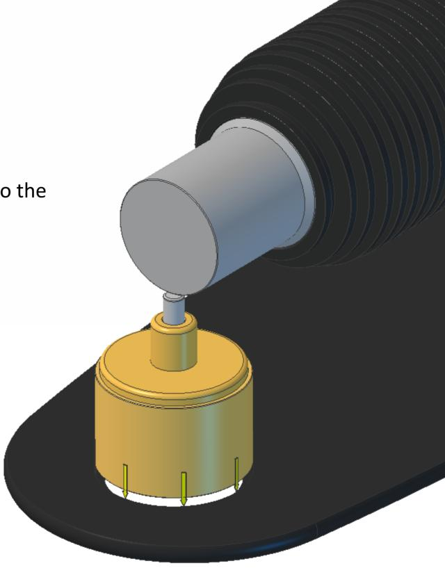
Light the wick and allow a minute or so to warm up. Press down on the engine above the foot to keep the engine still and spin the wheels.
