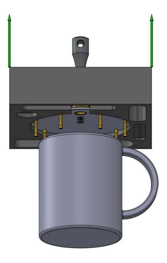
Hold the packing tray and engine firmly together so that the chamber pillars do not fall out of the top plate and remove the tray and engine from the mug.
