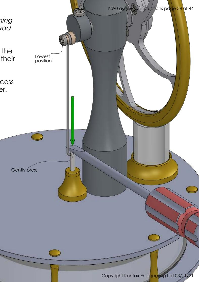
Slowly rotate the flywheel to move the displacer up and down in the chamber. Check that it does not touch the bottom plate. If it does touch you can go back and press the top of the gland stem a tiny bit more.
