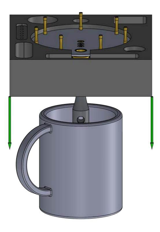
Still holding tray and engine firmly together carefully turn everything upside down and place back on top of the mug, with the main pillar inside the mug. The packing tray will hold the chamber pillars in a vertical position while you perform the next few assembly stages.
