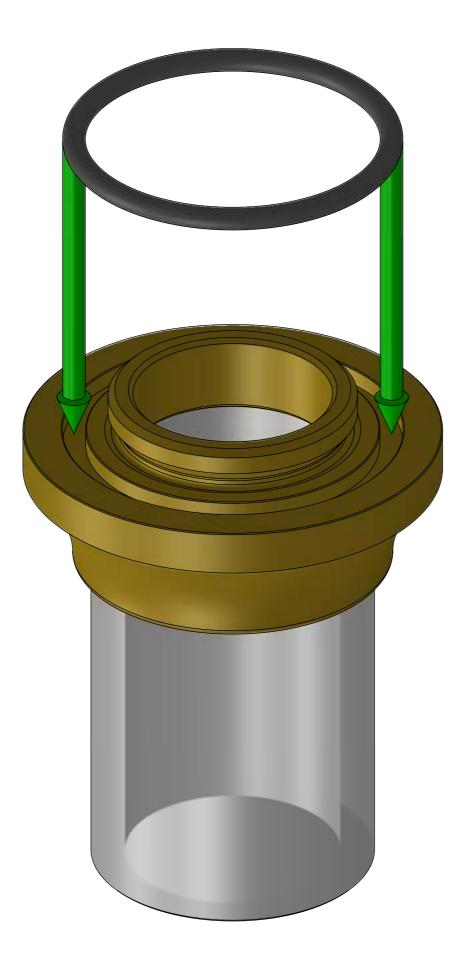
Screw the cylinder into the top side of the top plate and fully tighten, you might need to wrap an elastic band around it for grip. Make sure that the O ring does not become pinched or fall out of its groove. If you have trouble with the O ring falling out you can turn the plate upside down and screw the cylinder in from underneath.
