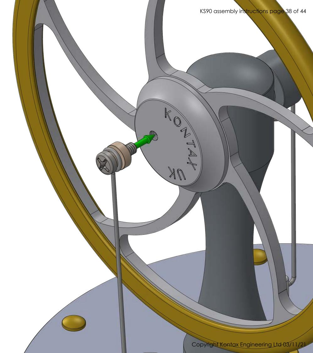
Your KS90 Stirling engine is now fully assembled. Check that the flywheel rotates fully and easily, a small amount of resistance will be felt on rotation due to the air pressure inside the main chamber. Re-check that the displacer does not bump into either plate. Once you have made these final checks you are ready to operate your engine.
