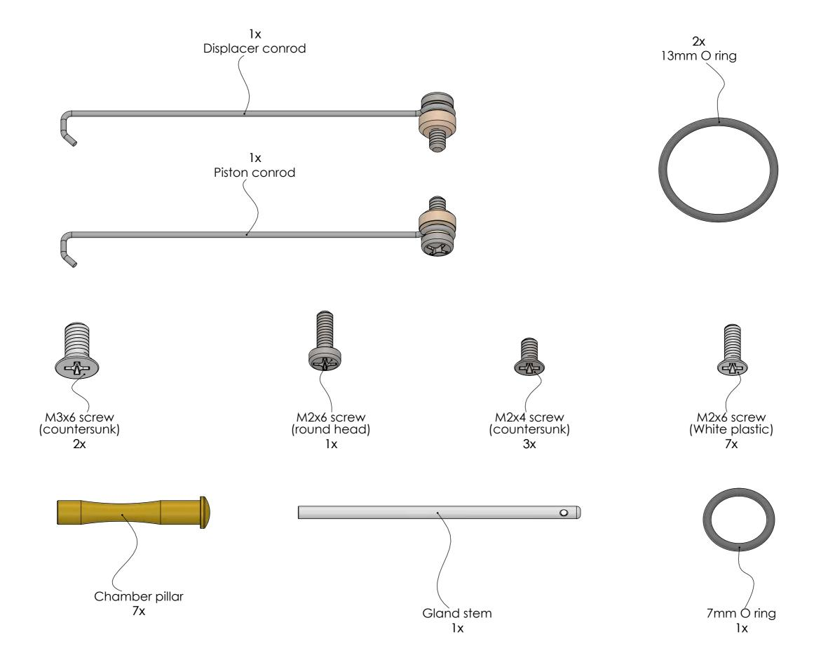
Fit one 7mm O ring into the groove in the bottom of the gland.
