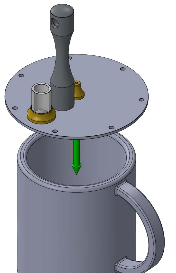
Remove the partially assembled engine from the packing tray and place it over the top of a coffee mug.
