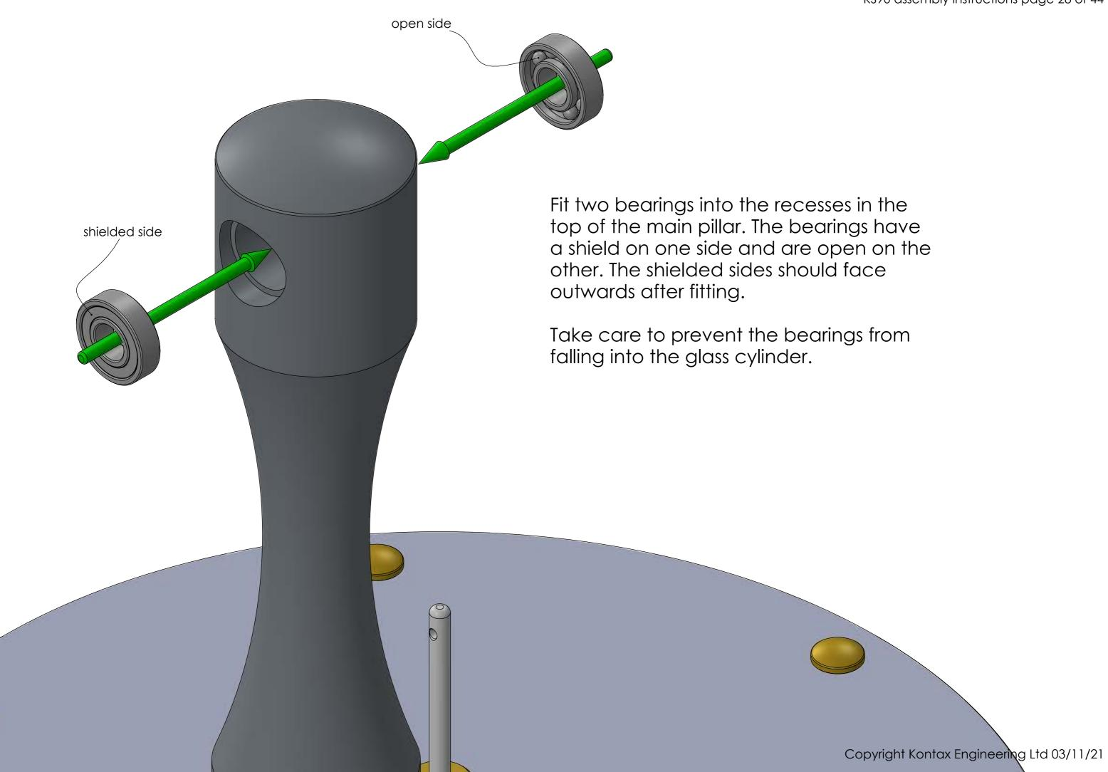
Slide the axle through the bearings. It should be a good fit but not tight in the bearings.
