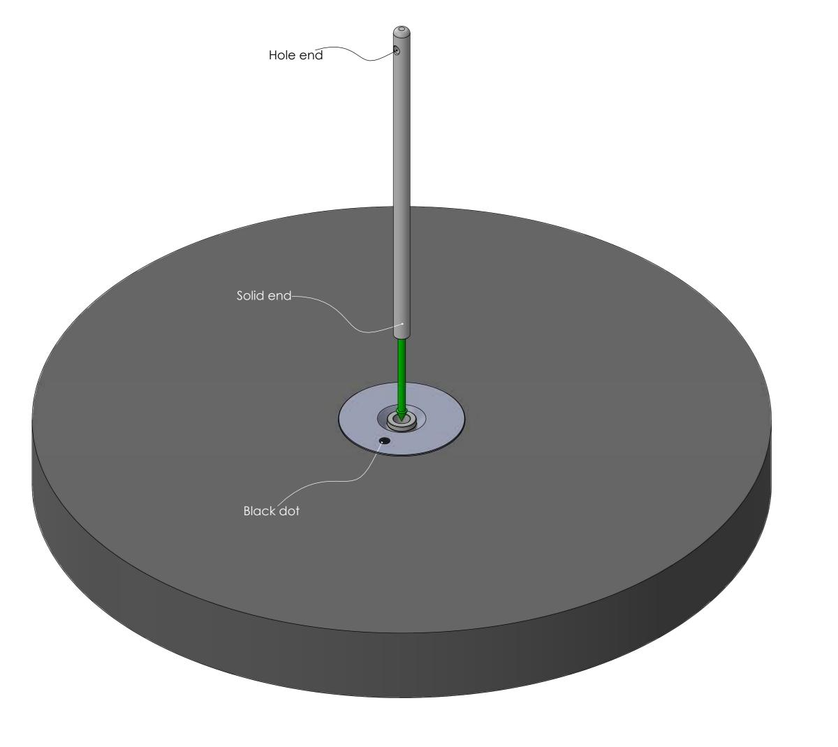
The top face of the displacer has been marked with a coloured dot near the centre.
