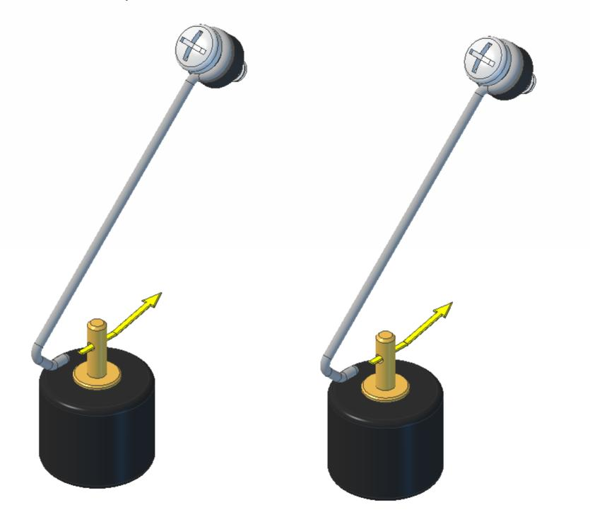
Slide one piston and conrod into the right hand cylinder. Some air pressure should be felt.
