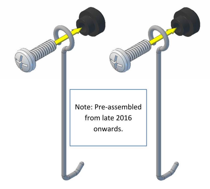
Screw the screws in until they *just* touch the bushes. Do not over-tighten or you could cause the bushes to expand and pinch the conrod eyes, which could prevent your engine from running.
