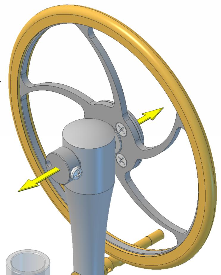
Give the flywheel a sharp spin; it should keep spinning for several minutes. If it does not then you will need to go back and move the crank out a fraction more. Fit one bearing bush, one ballrace bearing and one M2x6mm roundhead screw into the hole in the front of the crank. The shielded side of the bearing should face outwards after fitting. Fully tighten the screw.
