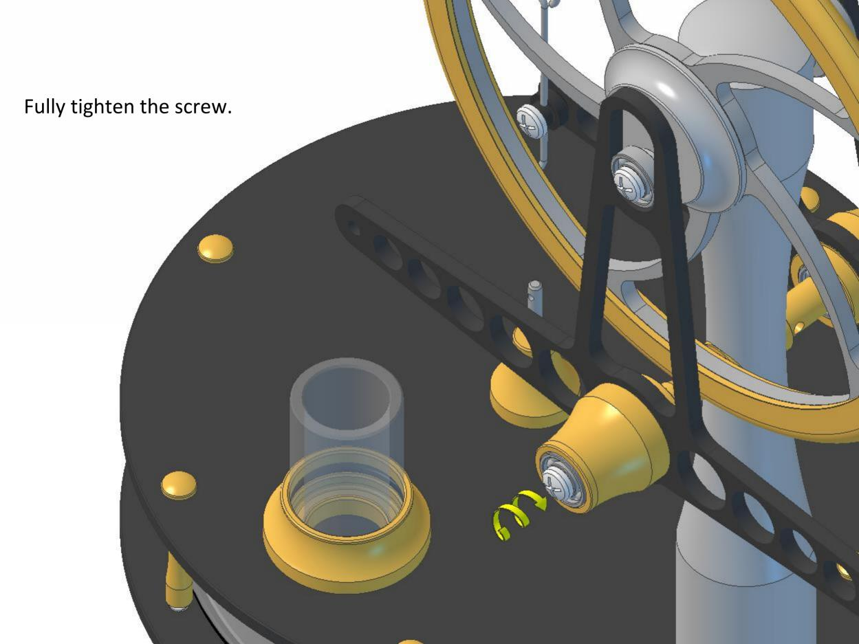
Fit one conrod onto one conrod bush and secure with one M2x6mm roundhead screw. The screw only needs screwing in a couple of turns at this stage. Note, the hook on the bottom of the conrod should be aligned as shown in the diagram. Repeat for the second conrod.
