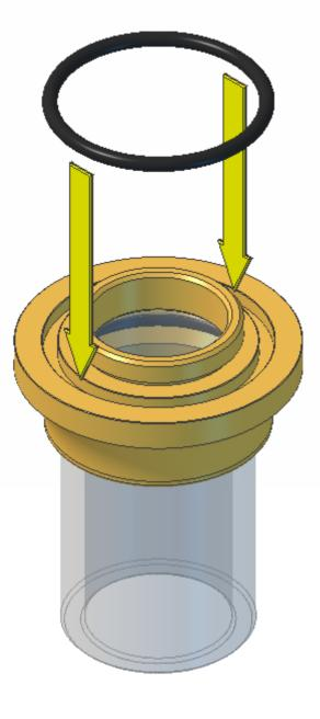
Insert two 13mm O rings into the grooves in the bottoms of the cylinders.
