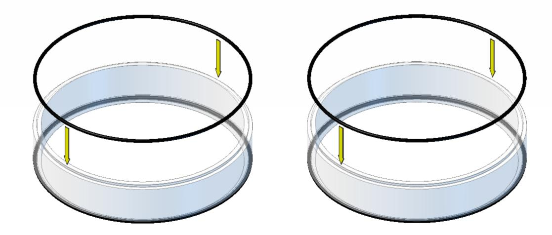
Lower each chamber wall and fitted O rings onto the upturned top plate. Make sure the O rings stay seated in their rebates, and that you do not dislodge any of the chamber pillars. The top faces of the displacers have been marked with a coloured dot near their centres.
