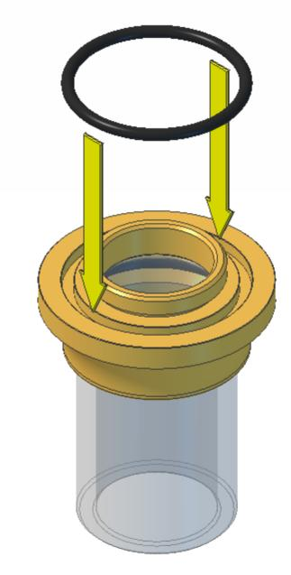
Screw the cylinders into the top plate and fully tighten, you might need to wrap an elastic band around them for grip. Make sure that the O rings do not become pinched or fall out of their grooves. If you have trouble with the O rings falling out you can turn the engine upside down and screw the cylinders in from underneath. Screw the front and rear T-bar carriers together through the hole in the main pillar.
