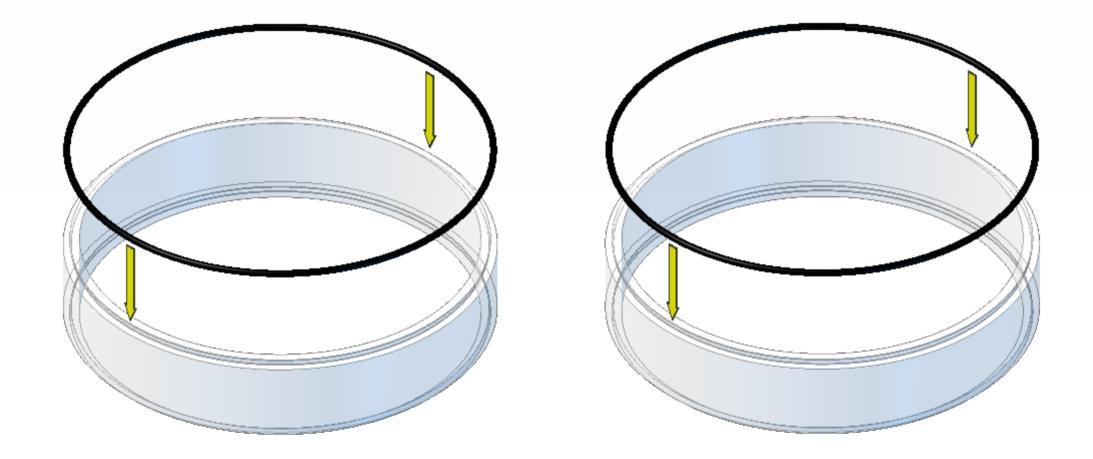
Stretch another 75mm O ring over the rebate on the other end of the first chamber wall. Repeat for the second chamber wall.
