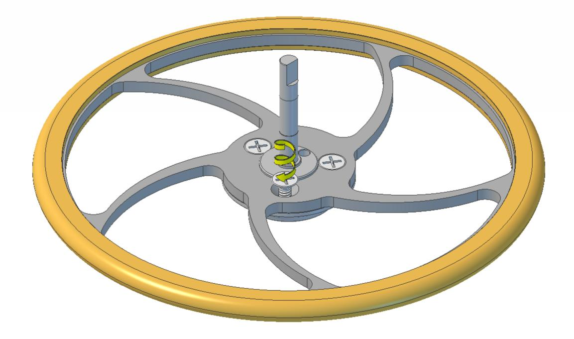
Slide the axle through the bearings. The axle should be a good fit but not tight in the bearings.
