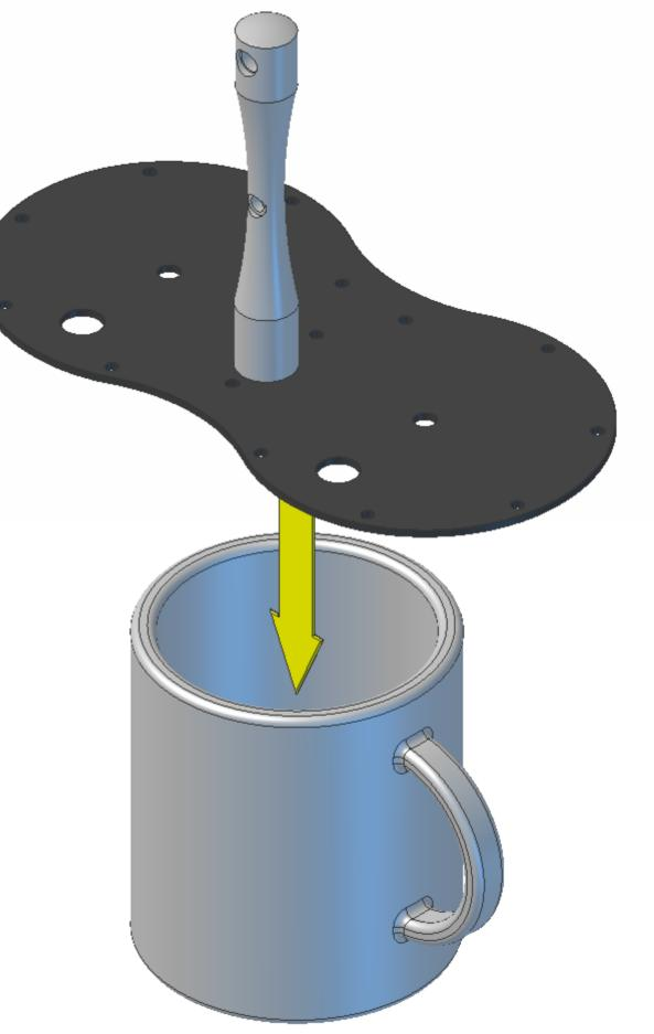
Insert fourteen chamber pillars into the fourteen small holes in the plate; they should all be an easy fit. If you have solar plates the heads of the pillars will sit <u>below</u> the surface, if you have polished or black plates the
