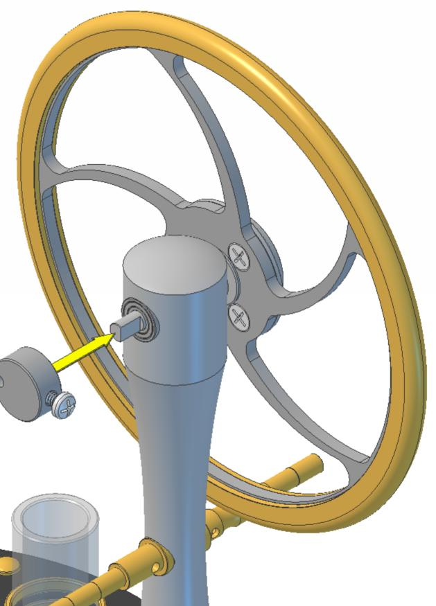
Make sure the crank screw is square on the axle flat, then fully tighten.
