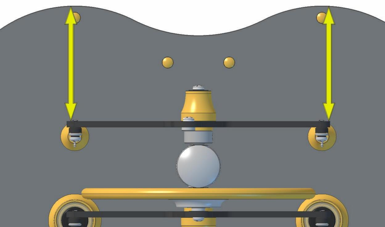
To adjust the alignment of the T-bar you will need to slacken the main pillar screws, adjust the T-bar and re-tighten the screws. Re-check and adjust until the T-bar is parallel.
