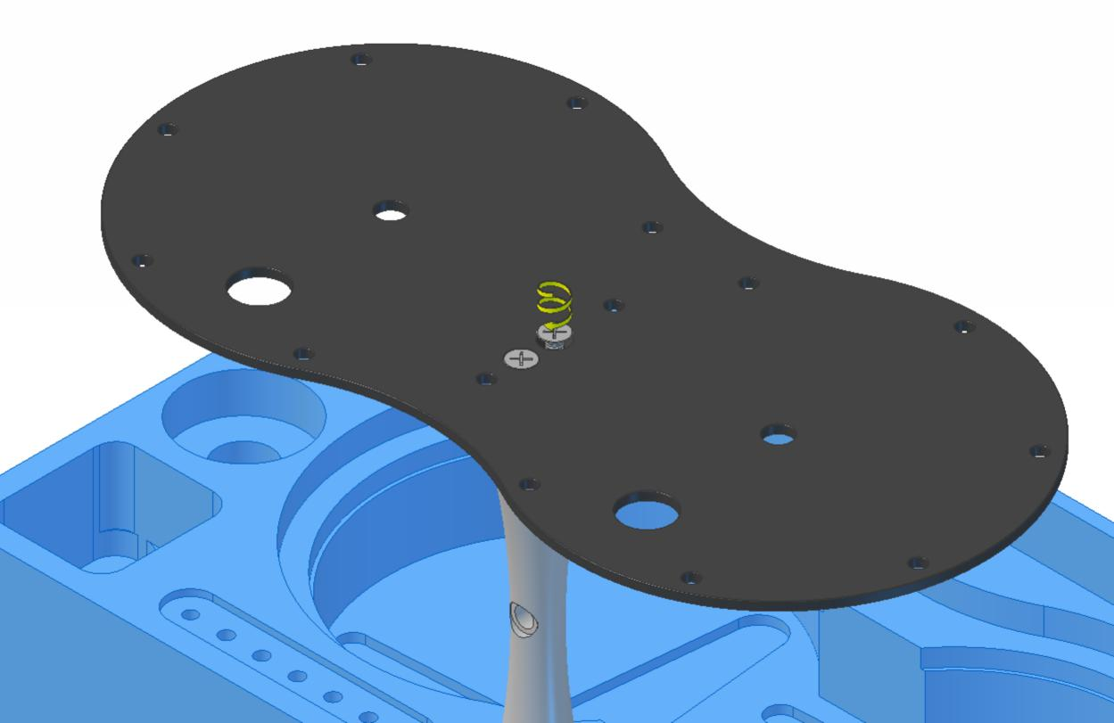
Remove the plate and pillar from the packing tray.
