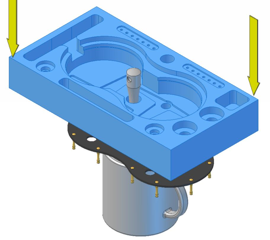
Hold the packing tray, mug and top plate firmly together so that the chamber pillars do not fall out of the plate. Carefully turn upside down and place on top of another two coffee mugs. Remove the top mug. The packing tray will hold the chamber pillars in a vertical position while you perform the next few assembly stages.
