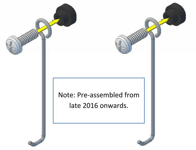
Screw the screws in until they *just* touch the bushes. Do not over-tighten or you could cause the bushes to expand and pinch the conrod eyes, which could prevent your engine from running.
