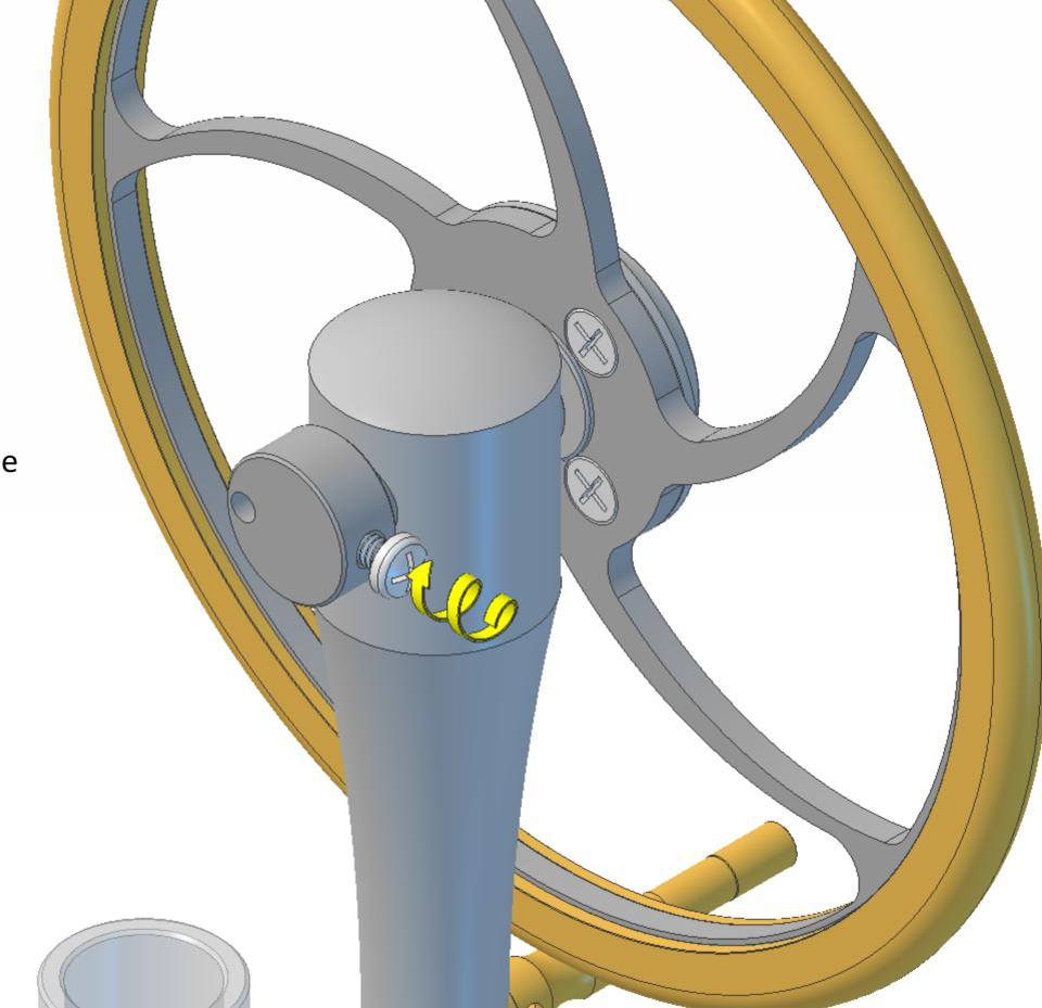
Gently push the flywheel back and forward, there should be a small amount of movement here. If there is not, slacken the crank screw, move the crank out a fraction and tighten. Make sure that when tightening the crank screw again it stays located on the small flat section on the axle.
