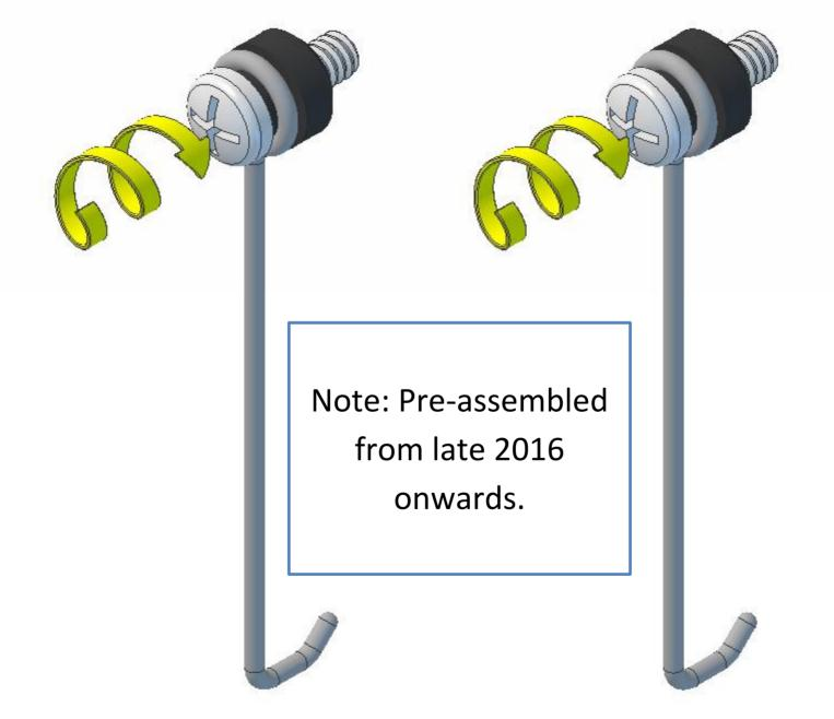
Fit the hook on the first conrod through the hole in the top of the first piston. Repeat for the second conrod and piston.
