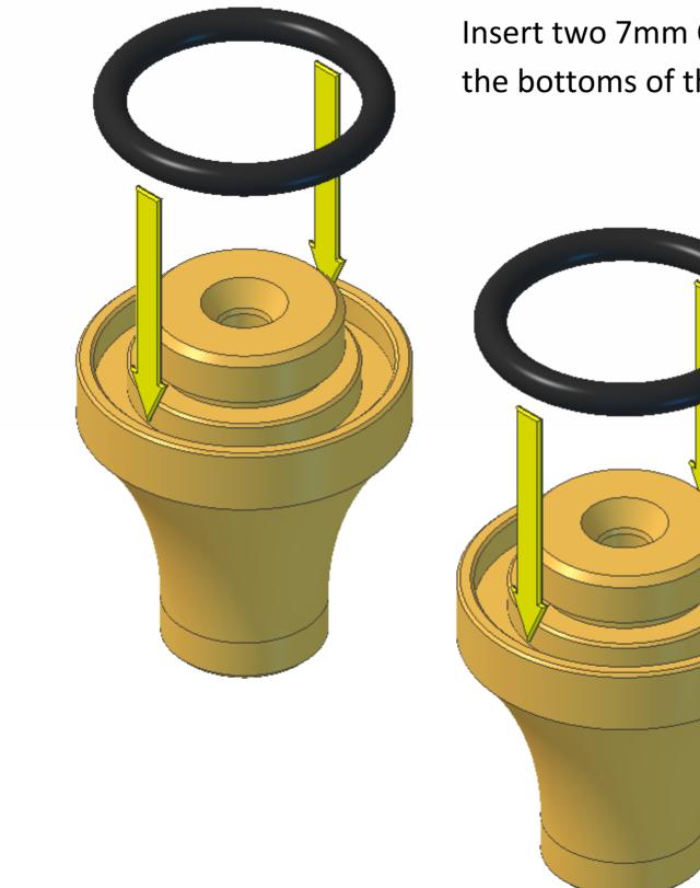
Insert two 7mm O rings into the grooves in the bottoms of the glands.
