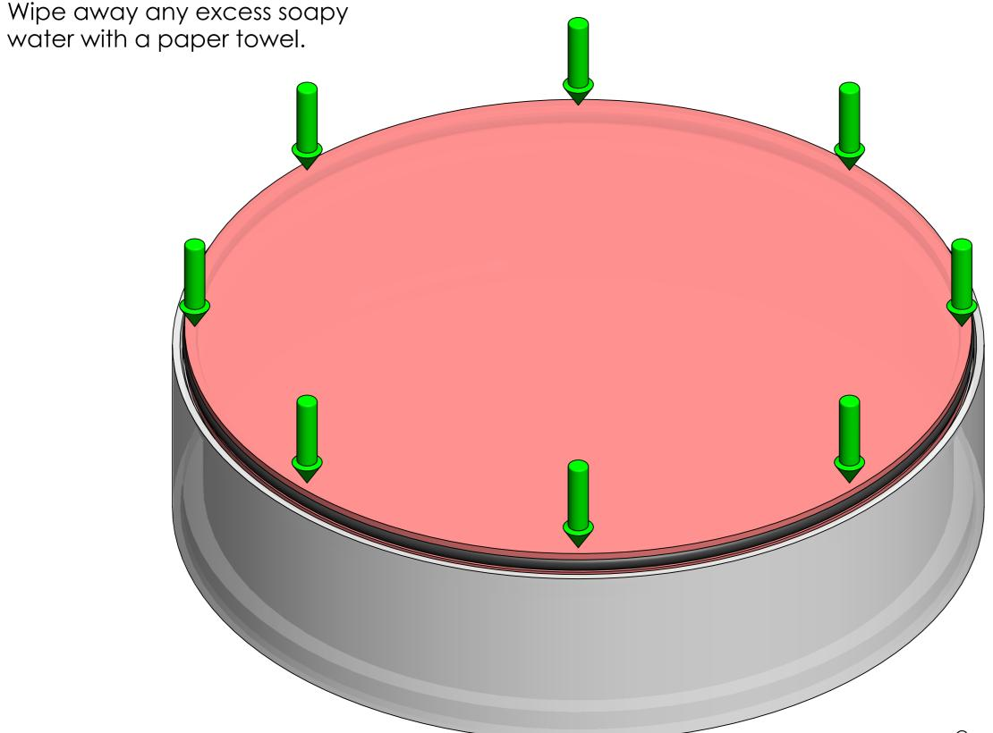
Check that the plate is pressed fully into the step on the wall.
