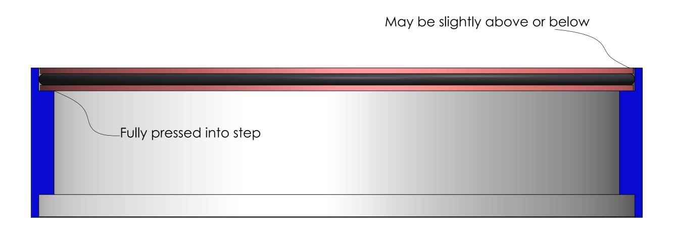
Fit one large O ring into the groove on the edge of the top plate, it will need a slight stretch to get it over the edge and into the groove.
