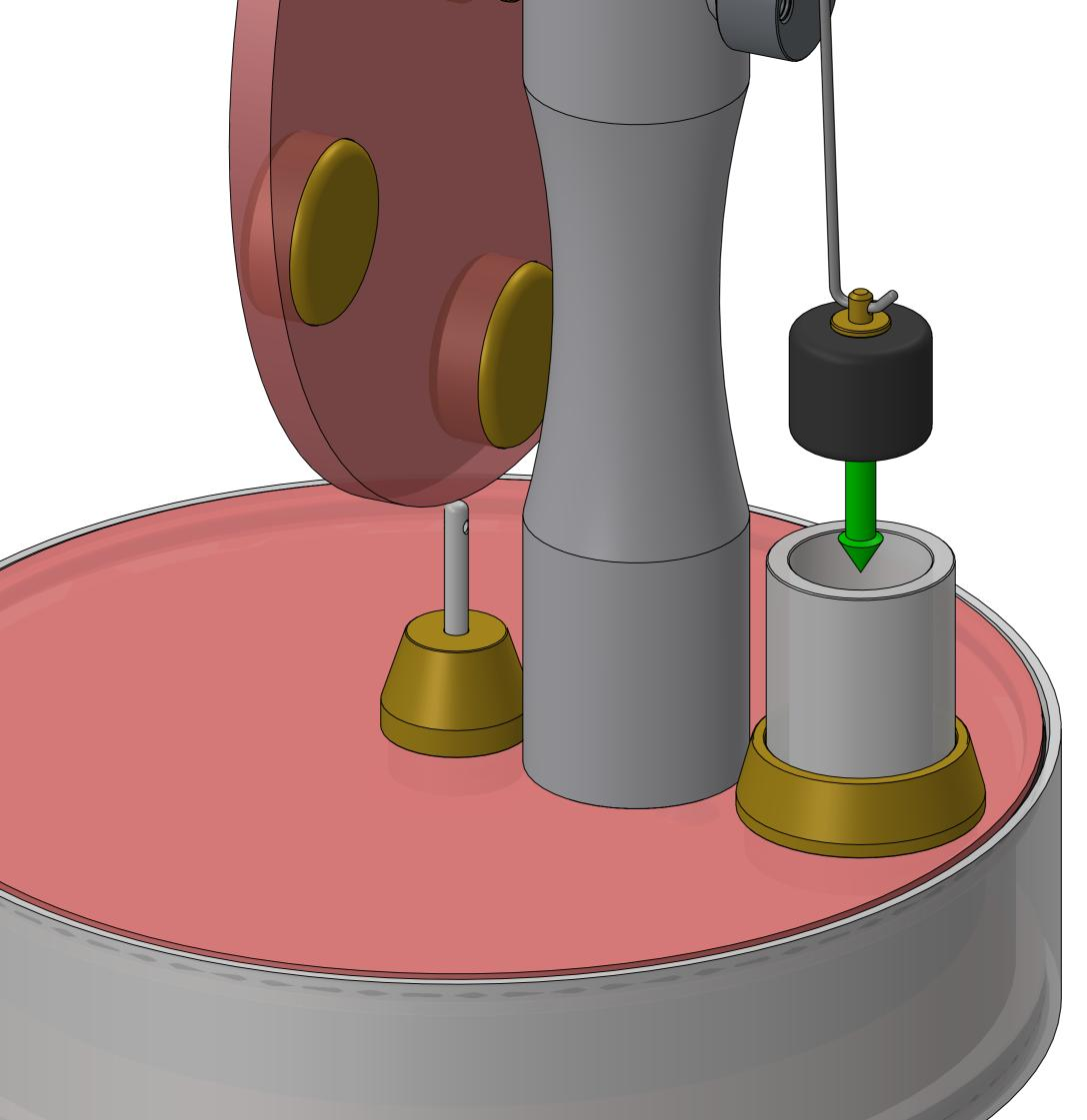
Slide the piston & conrod into the glass cylinder.
