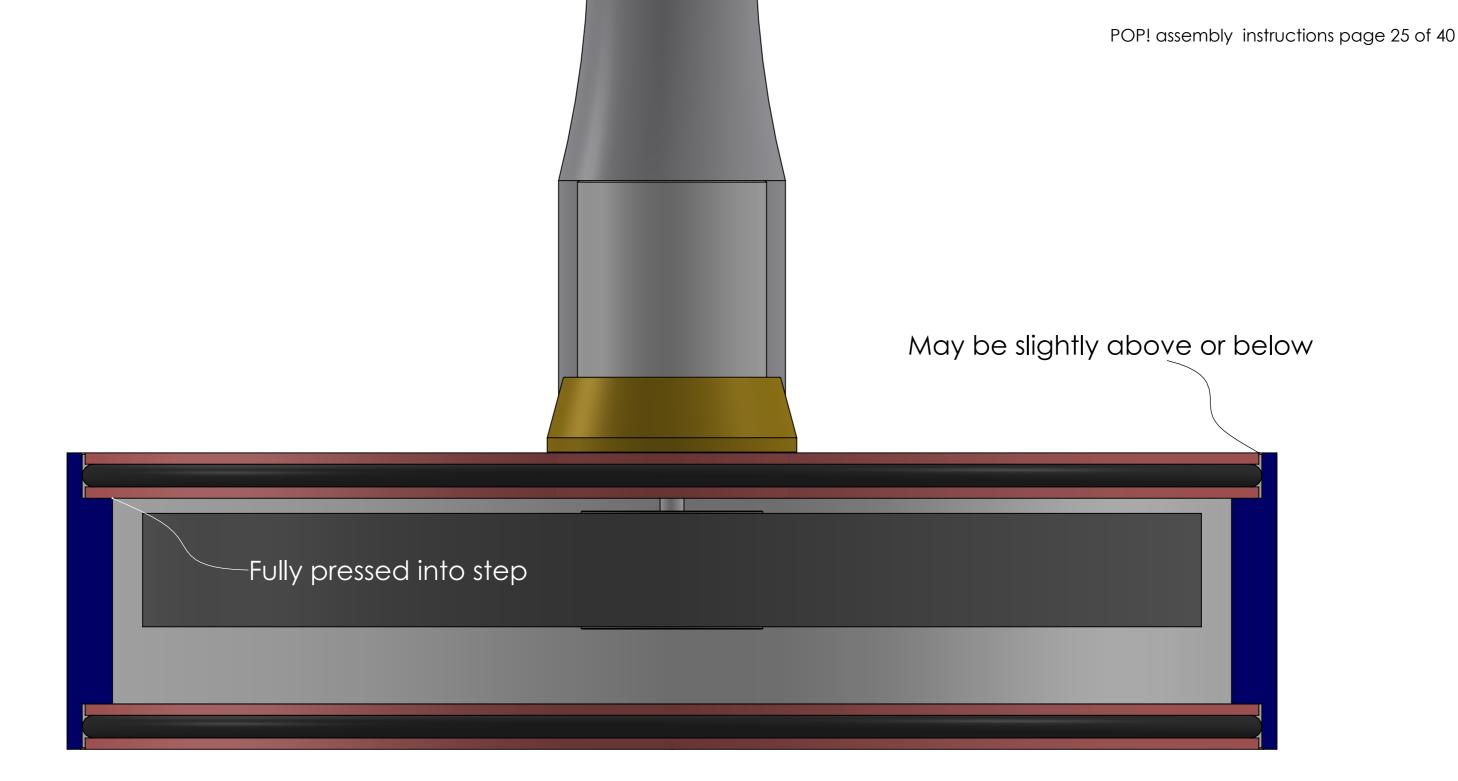
Check that the plate is pressed fully into the step on the wall.
