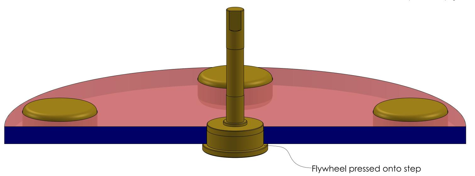
Check that the flywheel is correctly fitted onto the axle.
