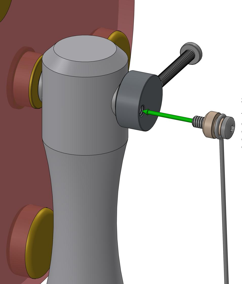
Screw the conrod screw into the crank.
