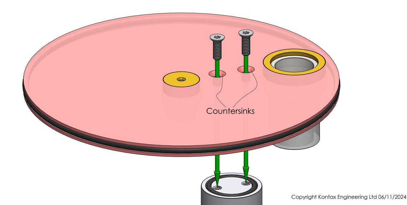
One end of the stem is solid and the other has a small hole through it.
