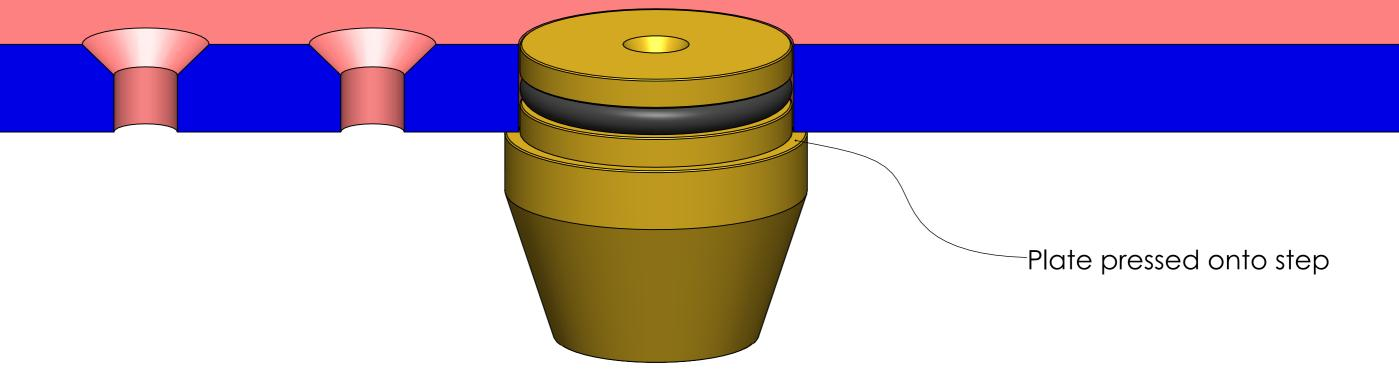
Check that the gland is correctly fitted into the top plate.
