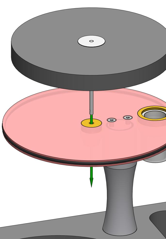
Slide the assembled displacer all the way into the gland.
