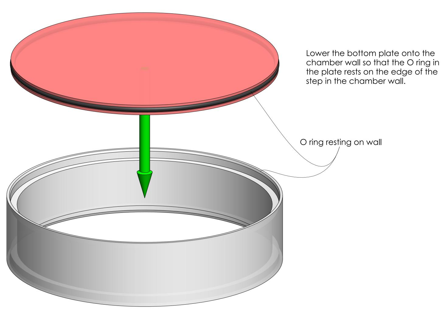
Spread your fingers evenly around the edge of the plate and gently press it into the step on the chamber wall, the O ring in the plate will squeeze into the step on the wall and provide an airtight seal between the plate and wall.
